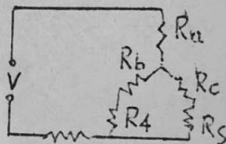
$$\text{onde } R_a = R_b = R_c = \frac{R_1 \times R_2}{R_1 + R_2 + R_3} = \frac{3 \times 3}{3 + 3 + 3} = \frac{9}{9} = 1 \Omega$$
