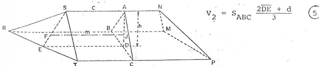
$$V_2 = S_{ABC} \frac{2\overline{DE} + \overline{d}}{3} \quad (5)$$
